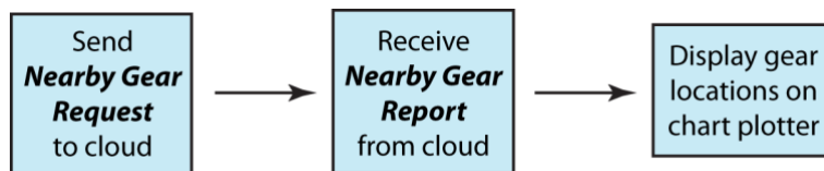
Figure 9. Flowchart initiated by Nearby Gear Request sent from a mobile fishing vessel (without an acoustic modem) to the cloud. The procedure used by the cloud to form the Nearby Gear Report is shown in Figure 10. The Nearby Gear Request is sent every 3 minutes from all ships. All of the procedures described here are controlled by the ship's command and control unit (CCU). The purpose of these procedures is to make available to a mobile vessel the location of fixed fishing gear in its immediate vicinity.
